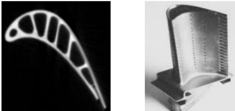
**FIGURE 1: Left – 2D CT slice of a turbine blade showing cooling passages. Right – external shot of a turbine blade showing cooling holes.**
