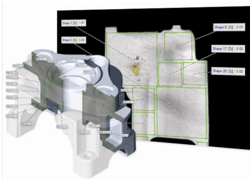
**FIGURE 3:** An example of porosity in a metal casting. The lower left corner shows CT scan data and the image to the right shows one cross sectional X-ray image that is highlighting various pores or holes that are internal to the casting.
