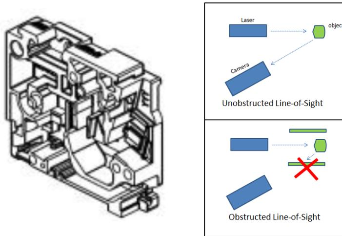
**FIGURE 2:** Left – an injection molded plastic part with high feature density. Right Top – Typical line-of-sight between the laser, the object being scanned and the camera. Right Bottom – An illustration of an obstructed line-of-sight.
